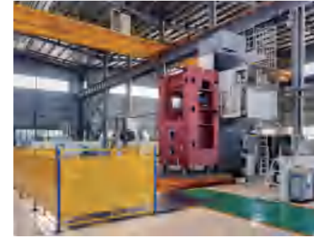
FBC160r数控滑枕剖台卧式铣镗床 FBC160r CNC horizontal ram milling and boring machine
