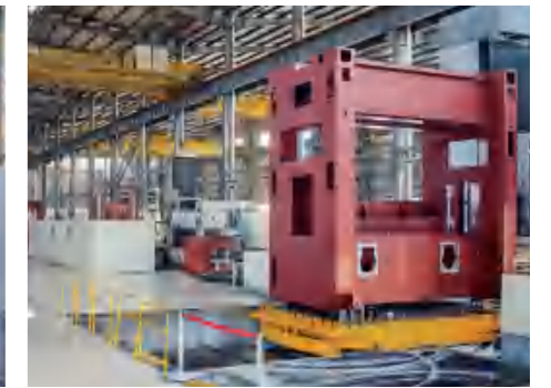
FBC160r数控滑枕剖台卧式铣镗床 FBC160r CNC sliding table horizontal milling and boring machine
